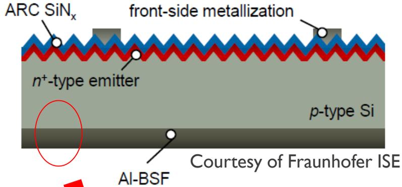
The whole rear silicon surface is in direct contact with Aluminium
