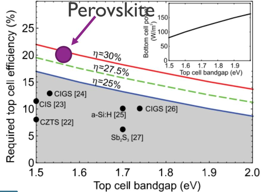
Needed: thin-film top cell with high bandgap, high efficiency, and minimal sub-bandgap absorption
