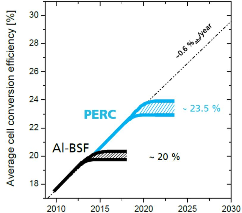
Further improvements possible by using passivating contacts, using to n-type silicon wafers and going to back-contact solar cells.
